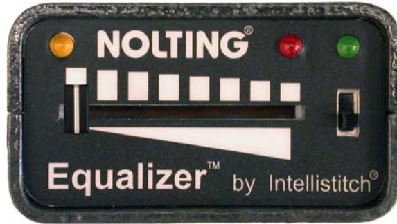
The green "RUN" light indicates that the machine is armed and ready to sew. The light flashes when the machine has not been moved for 4 seconds.
