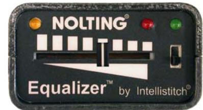
**To differentiate between the "up" and "down" positions a beep will sound when the needle is supposed to be at the "up" position.**
