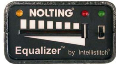
2. If the maximum speed needs adjustment, while still holding the RED BUTTON down, set the mode switch up if the speed needs to be increased, set it down if decreasing is necessary.
